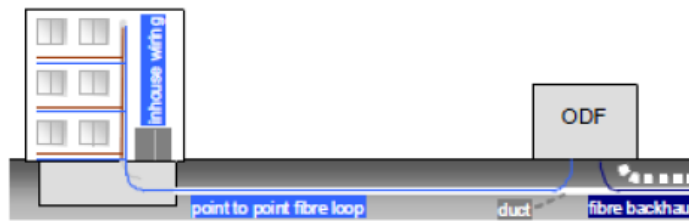
Point-to-point FttH design (BoR (10) 08, Ch. B.2.1.1)
